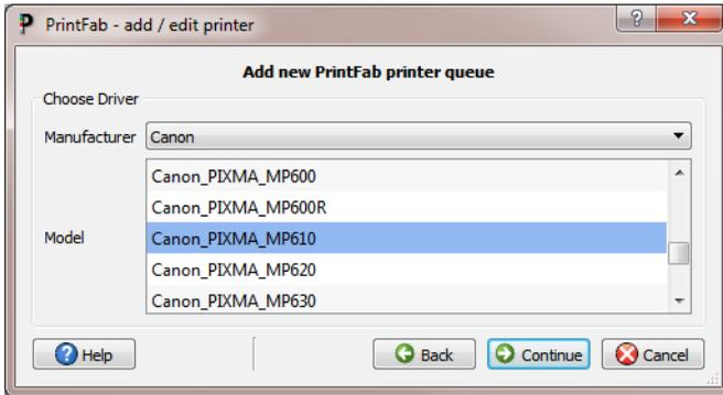
The next step is to enter a "**configuration name**" and a "**short name**" for the printer queue. In most application programs you can choose your printer using this configuration name.
